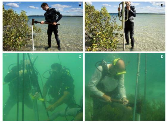
Figure 3.7 A demonstration of method used to drive corer into soil in seagrass meadows. (A) Shallow water with a sledgehammer (© Sarah Hoyt, Cl), (B) shallow water with a post-pounder (© Sarah Hoyt, Cl), (C and D) deep water with a sledgehammer (© James Fourqurean, FIU)
