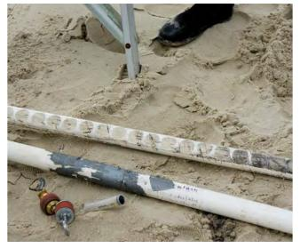
Figure 3.6 Seagrass coring devices. PVC tubes, rubber stopper, and syringe ( $\tilde{O}$  Cl/Sarah Hoyt)
