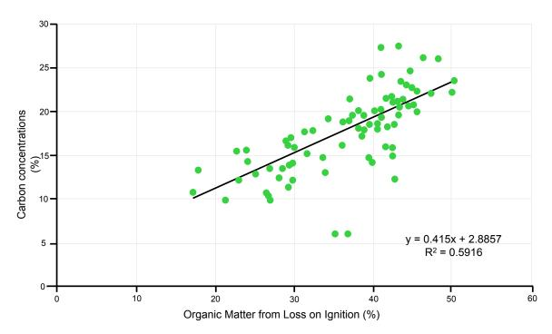
Figure D1 The relationship of organic matter calculated via loss on ignition to carbon concentration (percent) calculated via dry combustion for mangrove soil samples from the republic of Palau (Kauffman *et al.* 2011).
