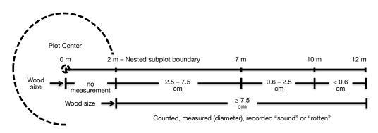
Figure 4.14 Example of a wood debris transect for sampling downed wood in mangroves using the line intersect technique. The diameter of each large wood piece encountered along the entire transect is measured. Smaller diameter pieces are counted but not measured along the designated lengths of the transect.
