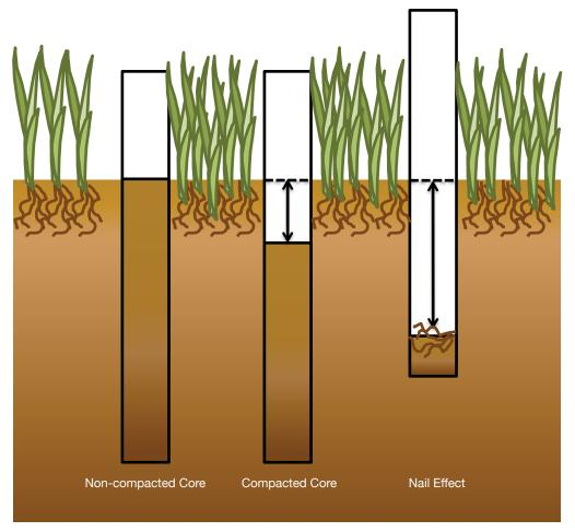
Figure 3.9 Diagram of soil core compaction that can occur while sampling. The top of a non-compacted core will be level with the surrounding ground (left). Cores can be compacted due to the force applied to the corer as it is driving into the soil (middle). The nail effect occurs when something (roots, rocks, shells, etc.) gets caught in the corer and compacts the soil underneath it (right).
