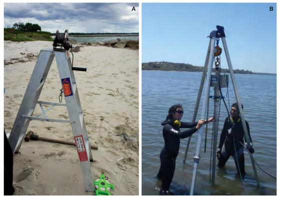
Figure 3.8 Set up for core sampling in seagrass ecosystems. Instruments for seagrass soil coring: (A) ladder with crank for removing coring device from soft soil in shallow water (© Sarah Hoyt, Cl), (B) sturdy tripod with weighted pulley system for removing coring device from soft soil in either shallow or deep water (© Oscar Serrano, ECU)
