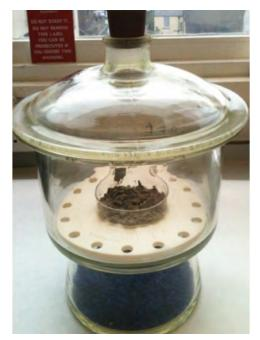
Figure 3.18 Soil sample cooling to room temperature in desiccator (© Hilary Kennedy, UWB)
