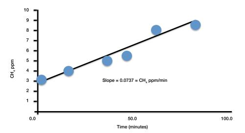
**Figure 5.6** Proportion of  $CH_4$  gas in the chamber is determined by plotting gas concentration per samples against the time between closing the chamber and collecting the sample. The slope is determined by calculating a best-fit line.
