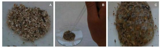
Figure 3.24 Testing for carbonate. (A) Subsample in a watch glass prior to acidification, (B) pipetting a few drops of weak HCl, (C) subsample effervescing. (© Hilary Kennedy, UWB)
