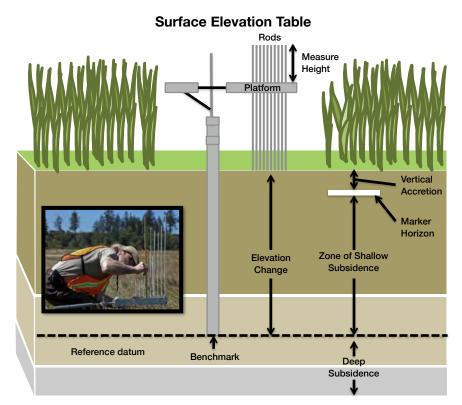
Figure 5.3 Diagram of a Surface Elevation Table (SET) marker horizon (MH) method used to detect changes in soil surface elevation. Inset image: USFWS biologist Bill Bridgeland taking measurements on a SET (© Roy Lowe, U.S. Fish and Wildlife Service).
