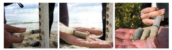
Figure 3.12 Cores are collected using a corer with predrilled sampling ports and sub-cores removed using cut-off polyethylene syringes (© Sarah Hoyt, Cl).
