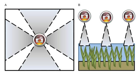
Figure 7.1 Photo point monitoring. (A) For mangrove plots, the person taking the photos stands in the center of the plot and takes a photo in each direction. (B) For seagrasses and salt marshes, photos are taken looking straight down and in various locations to get a general idea of the appearance of the site.
