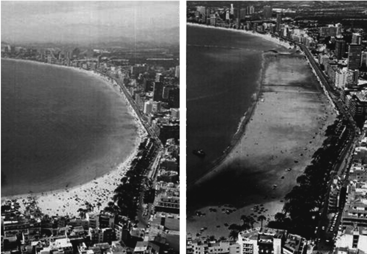
Fig. 2. Aerial image of Poniente Beach location before nourishment (left) and during nourishment (right) . Source: MOPT, 1991.
